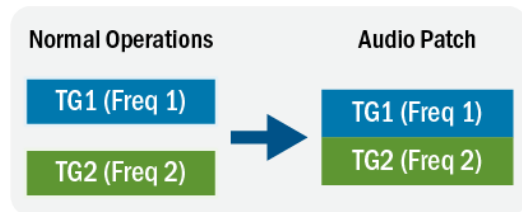
Figure 2 – Audio Patch of RF Resources
