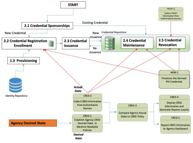
Figure 6-3: Credential Management Functional Block Diagram
