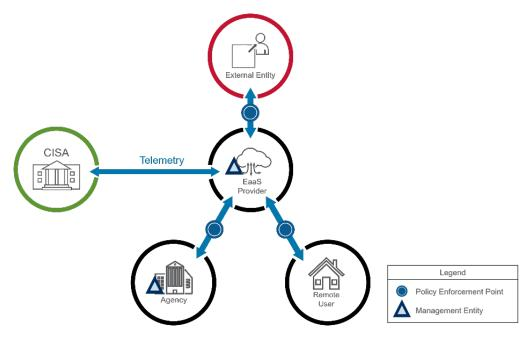
Figure 18: EaaS Telemetry Sharing with CISA
