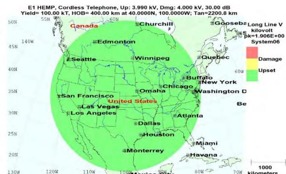
Figure 52. No cordless telephone damage with 30 dB protection
