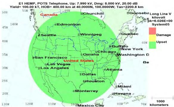
Figure 47. No POTS telephone damage with 20 dB protection
