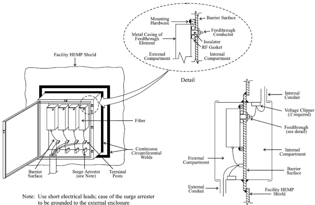
Figure 27. Typical cable POE protection design
