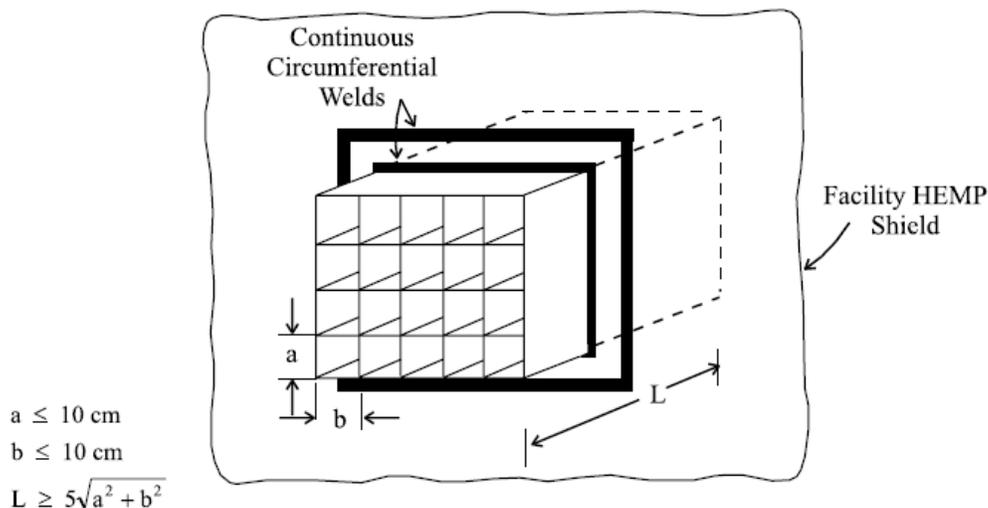
Figure 33. Typical waveguide-below-cutoff ventilation POE protective design for E1 HEMP <sup>15</sup>
