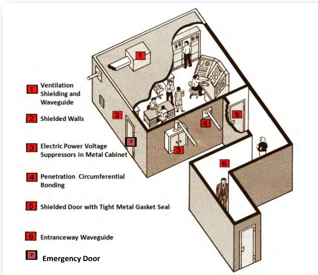
**Figure 26. Low-risk EMP barrier protection for facilities (per MIL-STD-188-125-1)**
