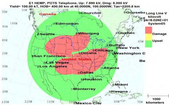
Figure 45. Devastating POTS telephone damage with 0 dB protection
