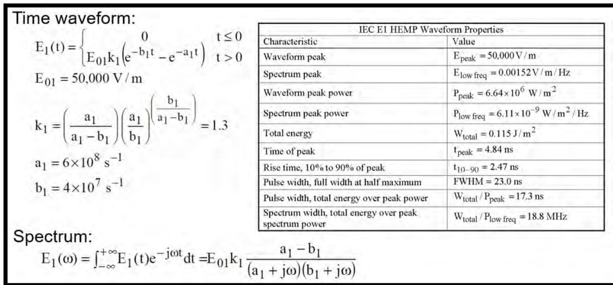
Figure 2. IEC Standard E1 Waveform (ref. IEC 61000-2-9)
