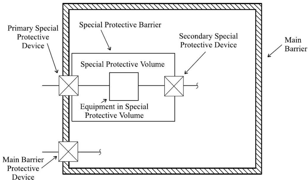
Figure 37. Special protective volume for electrical equipment
