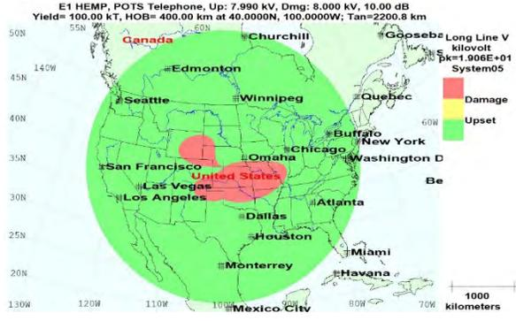
Figure 46. Significantly reduced damage with 10 dB protection
