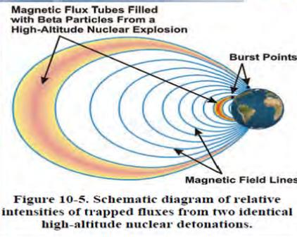
Figure 10-5. Schematic diagram of relative intensities of trapped fluxes from two identical high-altitude nuclear detonations.
