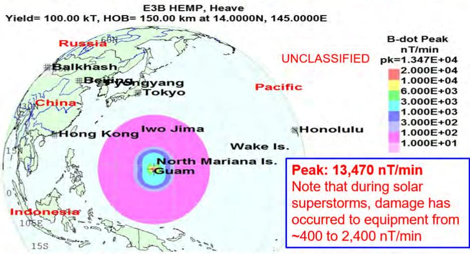
Above: A 100 kT “generic” nuclear weapon detonated at 150 km altitude above Guam could generate a powerful low frequency “heave” E3B pulse that could couple into power lines and other long conductors, such as undersea cables. This graphic shows that Guam is covered by significant, low frequency EMP for a period of up to 300 seconds after the burst (at levels up to a maximum of 13,470 nanoteslas/minute).
