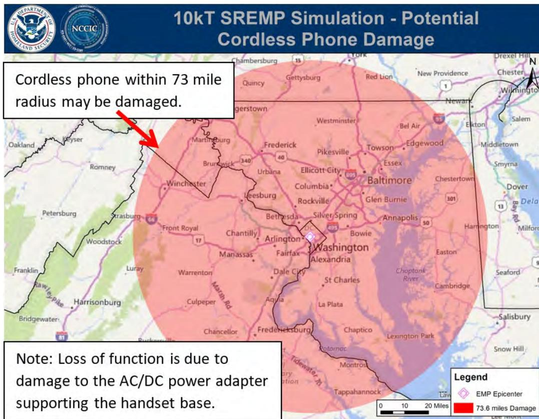
Figure 13. Potential 10 kT SREMP disruption of AC/DC adapters
