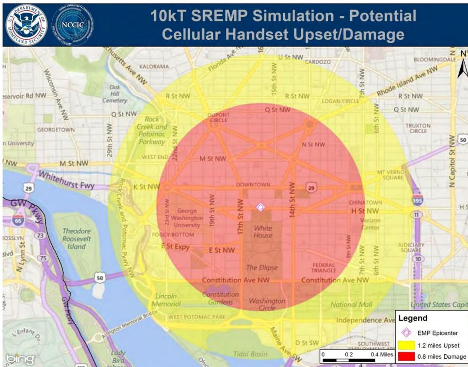
Figure 15. Potential 10 kt SREMP Upset/Damage to Cellular Handsets
