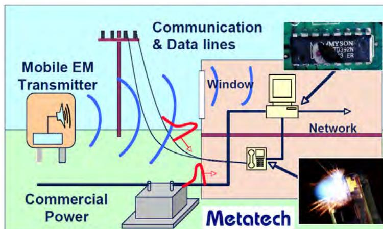
Figure 16. Typical IEMI interaction of radiated fields
