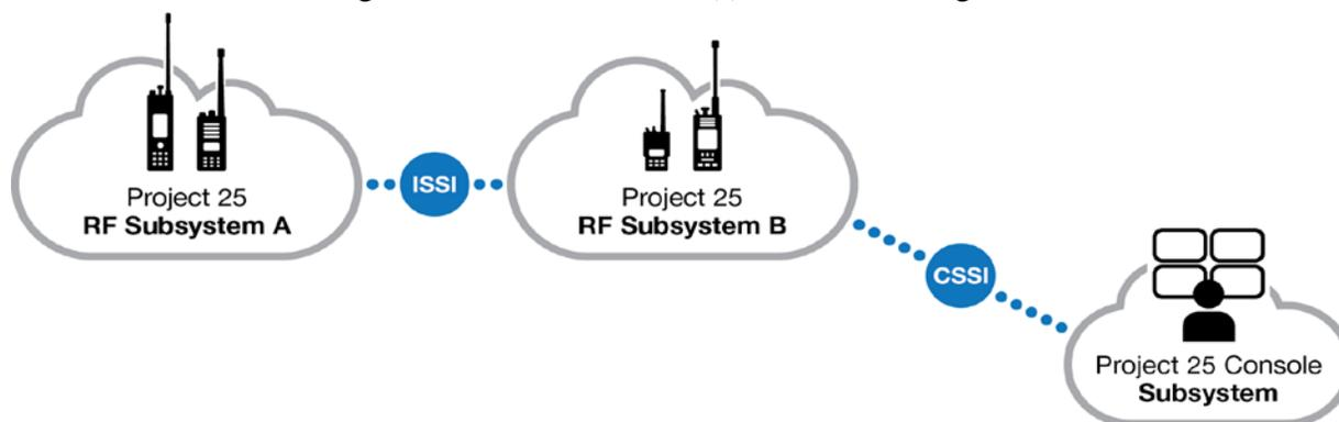
Figure 1. Connecting RF Subsystems Using ISSI and CSSI.
