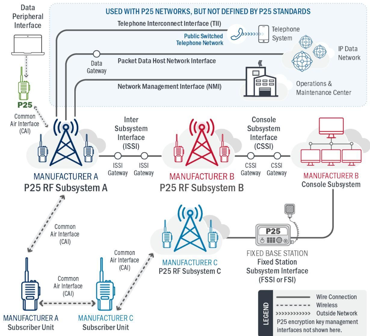
Figure 1: P25 System Model
