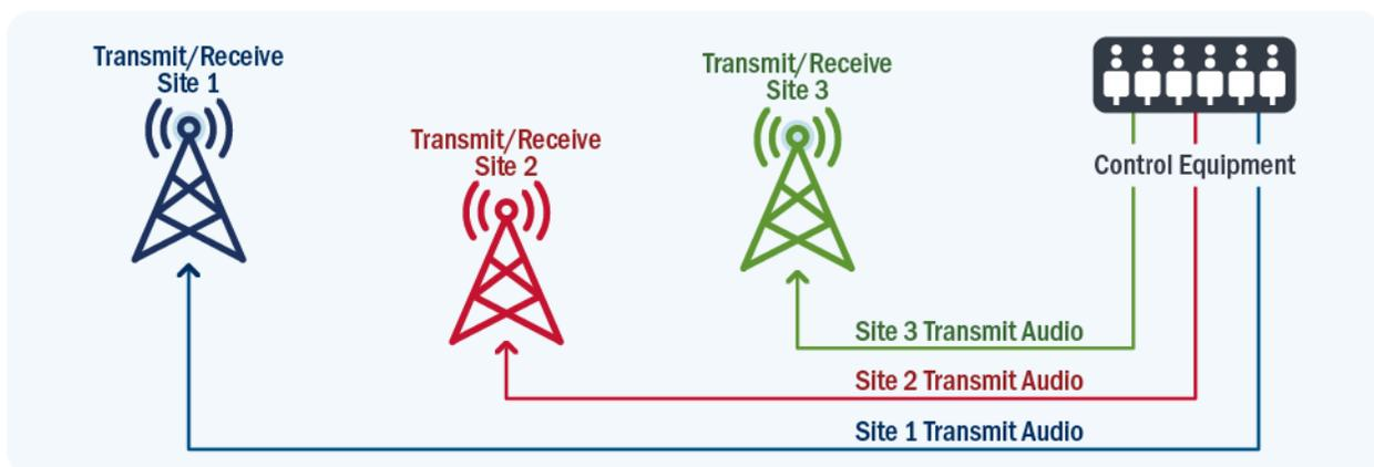
Figure 10: Simulcast Voting Example. In this diagram, signals received at multiple sites are sent to the control equipment, where a voting comparator chooses the best signal to rebroadcast across the system.
