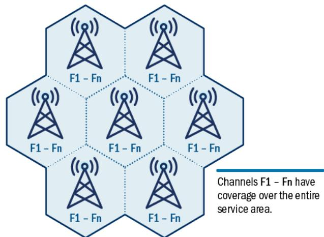
Figure 8: Simulcast Layout
