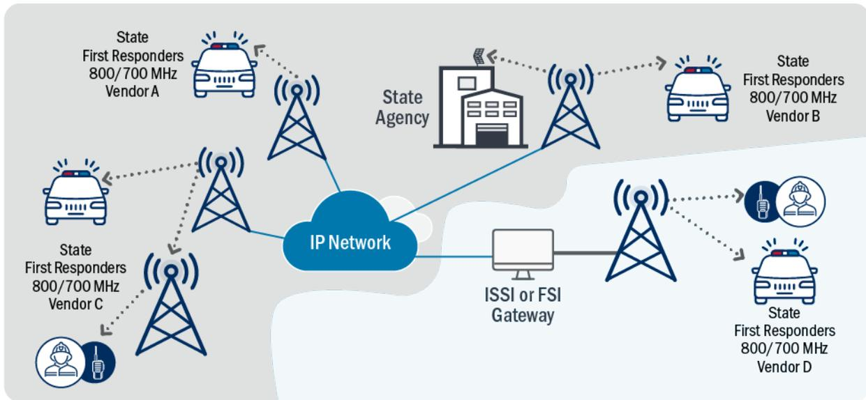
Figure 7: Wide Area P25 Network with IP Backhaul
