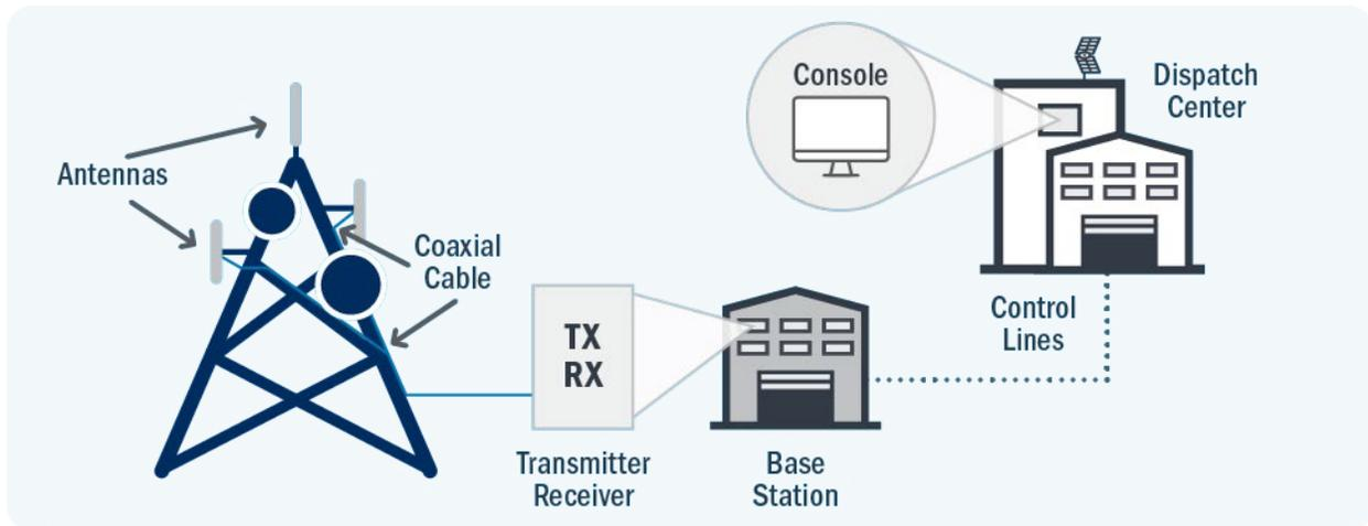
Figure 17: Console Subsystem Connected to Base Station
