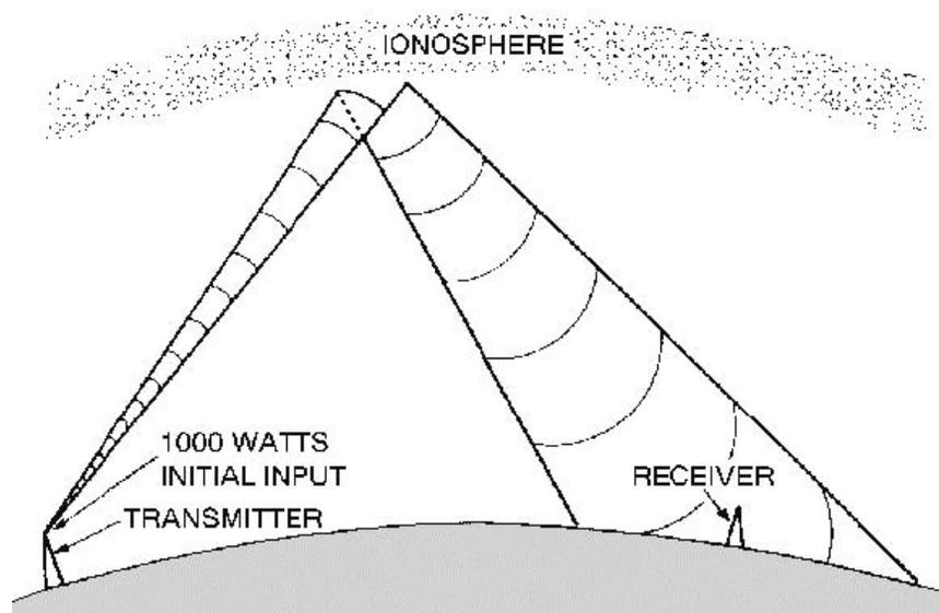
Figure 1-14.—Free space loss principle.
