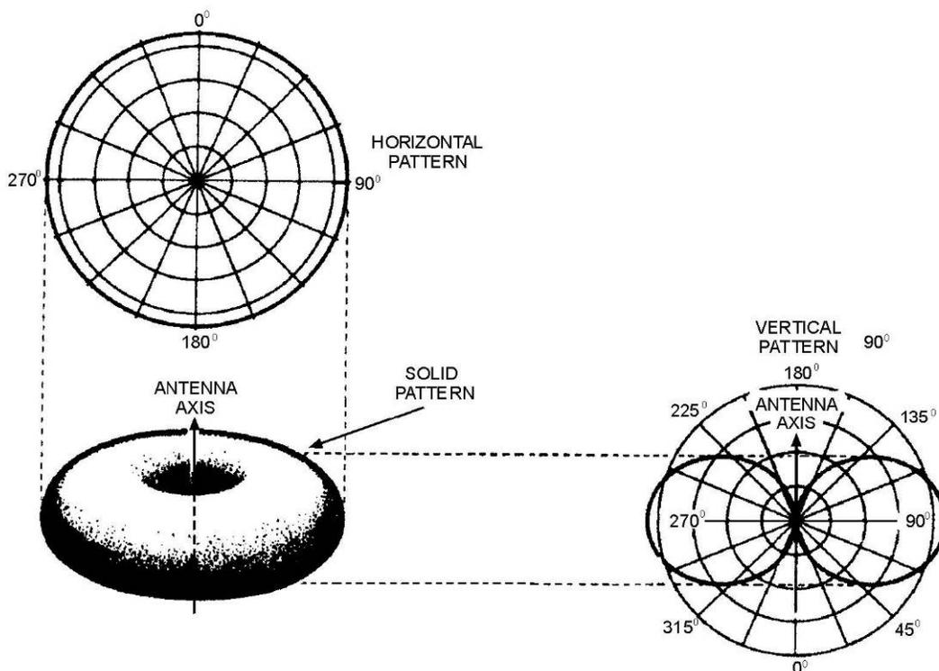
Figure 1-29.—Radiation pattern of a dipole.
