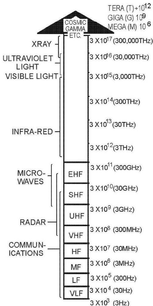
Figure 1-1.—Electromagnetic spectrum.
