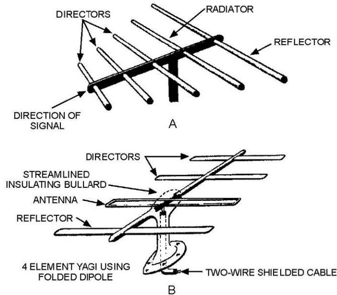
**Figure 1-37.—Yagi antenna.**
