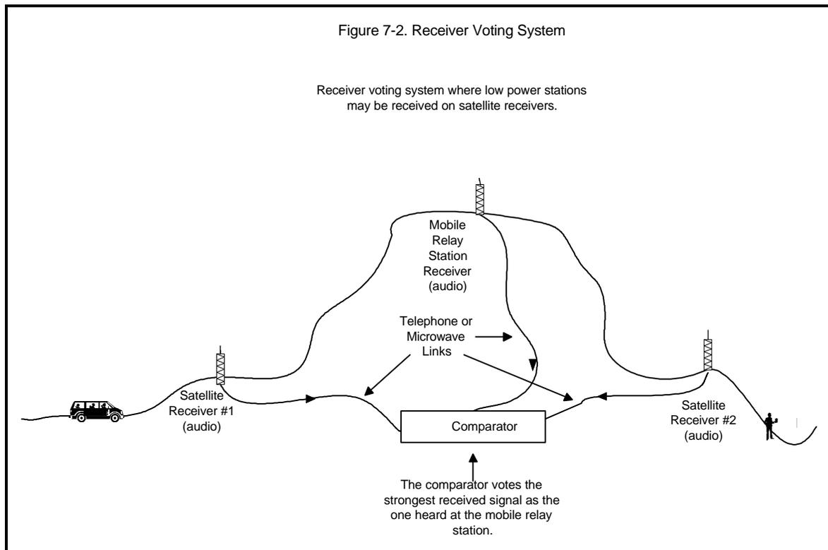
Another scheme used where there are problems transmitting to and receiving from mobiles and handheld radios due to large changes in topography requires several repeaters at different locations that may be switched at a central position, usually at the police communications dispatch center, to the repeater receiving the highest signal level. In this way the signal is "steered" toward the station, as shown in figure 7-3.
