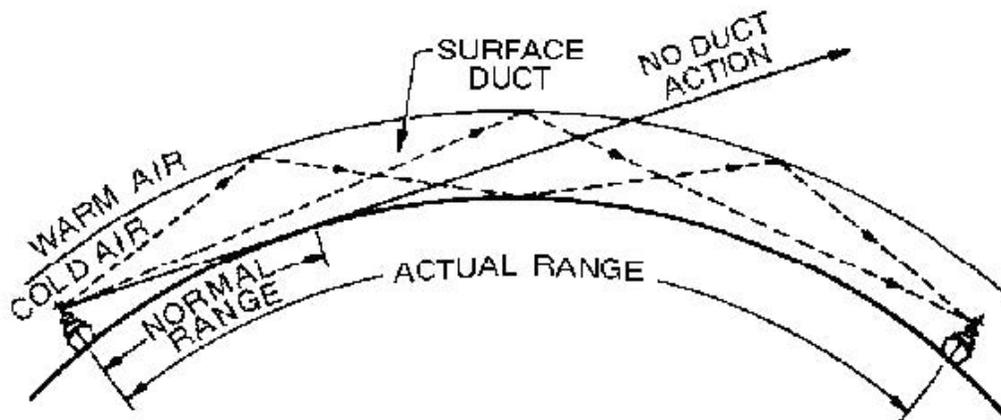
Figure 1-16.—Duct effect caused by temperature inversion.
