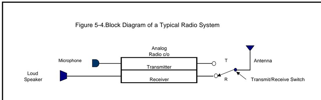
An analog system may also carry data. However, the data, which are in digital form of binary digits, or bits (i.e., ones and zeros), must first be converted to an analog signal. A modem (modulate/demodulate unit) is used to convert the ones and zeros into two analog tones representing either a one or a zero. When the analog data arrive at the receiver, they are converted back to digital form again using another modem.
