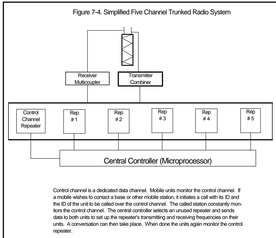
When it issued rules for the 800 MHz band, the FCC required that most licensees requiring five or more channels *must* use a trunked radio scheme.<sup>4</sup> Systems in place before the regulation was issued are "grandfathered in" and may continue to add single repeater stations as necessary.
