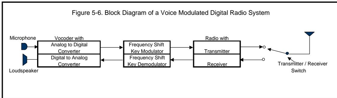
A digital radio system transmits data directly, by digitally modulating a carrier. One simple method of modulation is to change the carrier frequency by shifting it different amounts for each type of bit. (This is called *frequency shift keying*, or FSK.) The receiver then receives the signal as a zero or as a one and re-creates the original signal.
