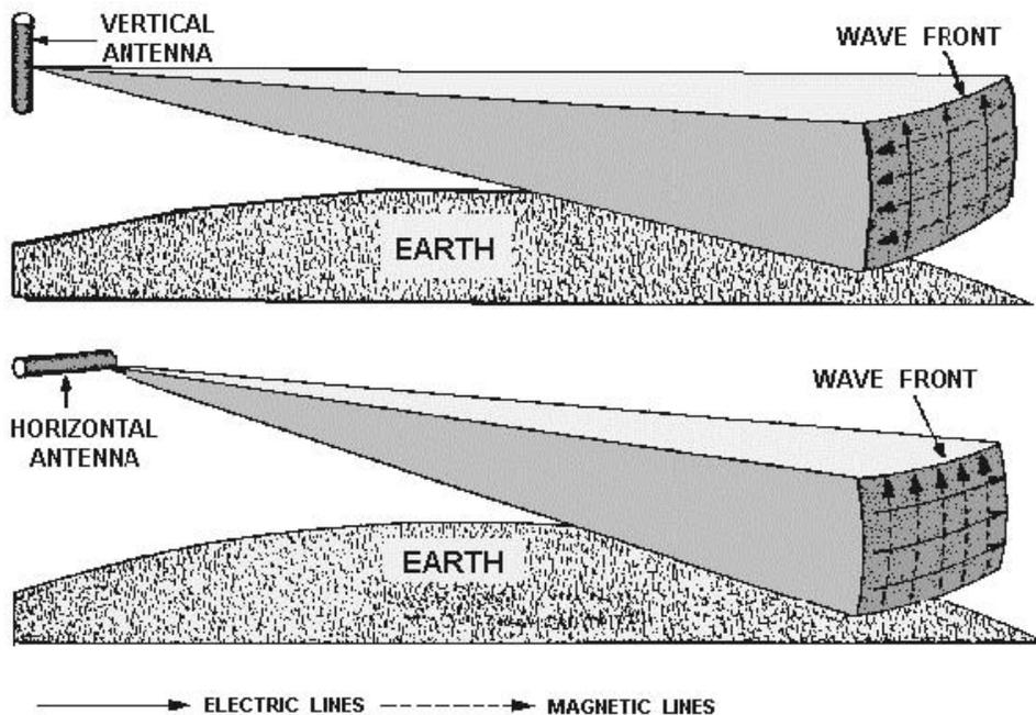
Figure 1-4 Polarization.
