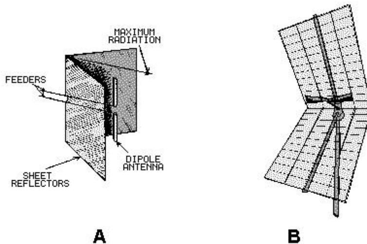
Figure 1-39.—Corner-reflector an
