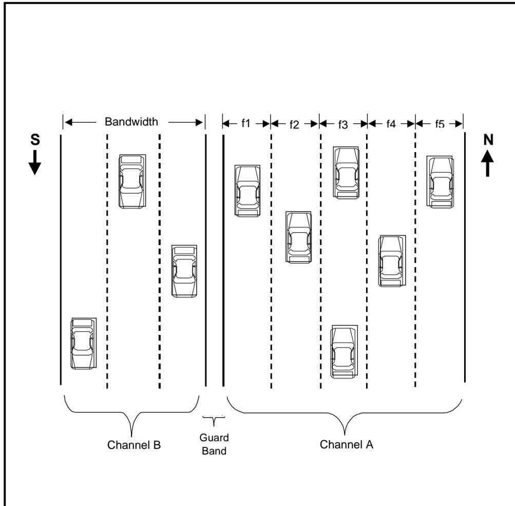
In a similar way, a second channel could be compared to the other side of the highway where all of the lanes travel in a different direction (southbound). A concrete barrier or median strip exists to separate the northbound lanes from the southbound lanes. A similar non-overlap space exists between channels and is called the *guard band*.
