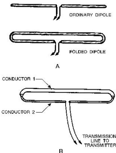
**Figure 1-33.—Folded-dipole antennas.**
