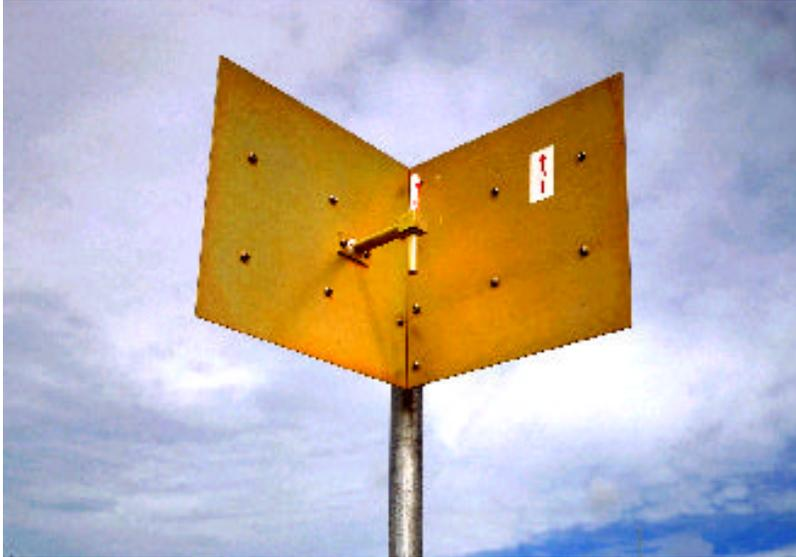
Figure 6-12. Yagi Antenna
