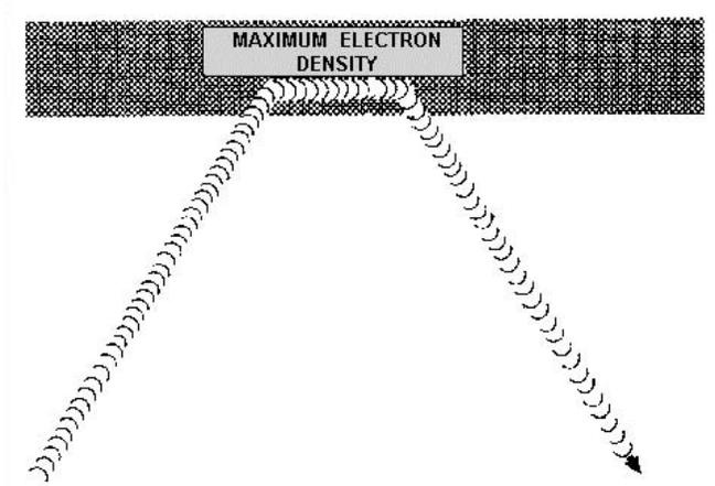
**Figure 1-6.—Radio wave refraction.**
