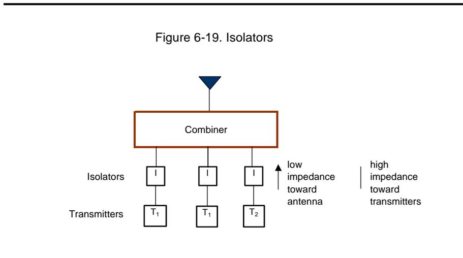
If there is inadequate isolation, the mixing of the transmitted signals can cause the generation of additional frequencies called intermodulation products, or IM products, which may cause interference to nearby receivers.
