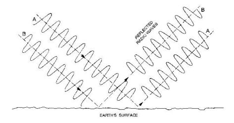
Figure 1-5.—Phase shift of reflected radio waves.
