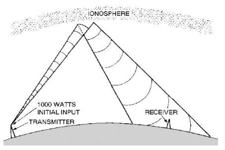
Figure 1-14.—Free space loss principle.
