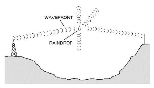
Figure 1-15.—Rf energy losses from scattering.
