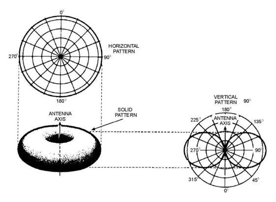
Figure 1-29.—Radiation pattern of a dipole.
