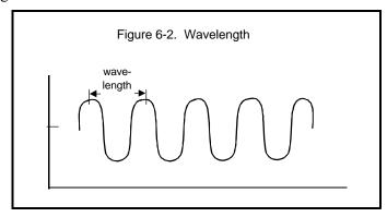
In radio terms, a *short* wavelength would mean that the peaks are relatively close together. A *long* wavelength would mean that the peaks are relatively far apart.
