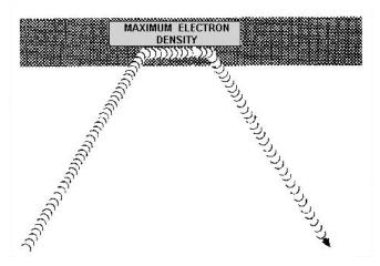
Figure 1-6.—Radio wave refraction.
