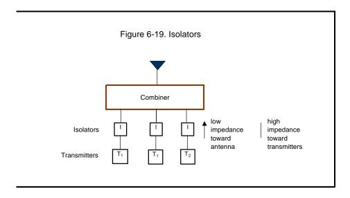
If there is inadequate isolation, the mixing of the transmitted signals can cause the generation of additional frequencies called intermodulation products, or IM products, which may cause interference to nearby receivers.
