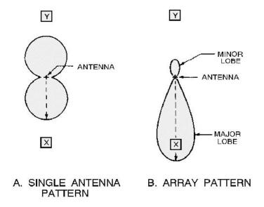
Figure 1-35.—Single antenna versus array.
