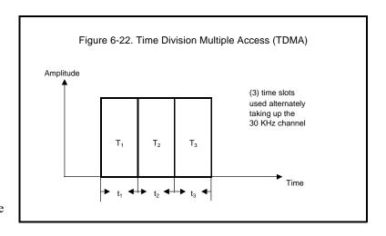
Group of special mobile (GSM), which was developed in Europe and is being used by a number of U.S. companies, provides TDMA transmission with 200 KHz wide channels in the 2 GHz band.
