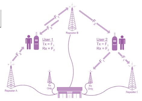
Figure 16-7: Simulcast Repeaters with Remote Receivers
