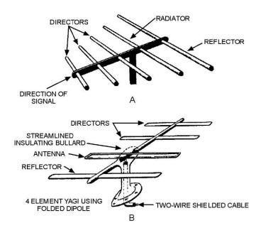
Figure 1-37.—Yagi antenna.
