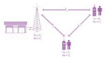
Figure 16-4: Simplex Radio Example
