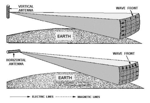
Figure 1-4 Polarization.
