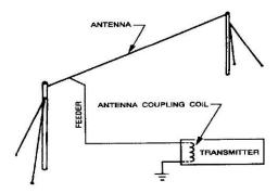
Figure 1-25.—Typical antenna system.
