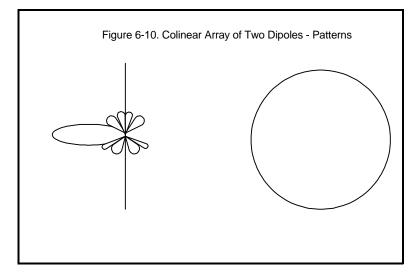
left side of figure 6-10. The side lobe amplitudes are much less than that of the main lobe. The beam width of the main lobe is defined as the angle between the half power points.
