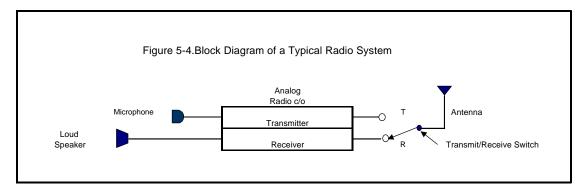
An analog system may also carry data. However, the data, which are in digital form of binary digits, or bits (i.e., ones and zeros), must first be converted to an analog signal. A modem (modulate/demodulate unit) is used to convert the ones and zeros into two analog tones representing either a one or a zero. When the analog data arrive at the receiver, they are converted back to digital form again using another modem.
