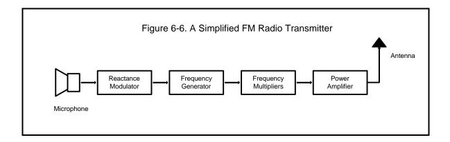
The output frequency is a continuous wave (CW) called a carrier. Intelligence is added to the transmitter by varying the *amplitude* of the carrier (amplitude modulation or AM) or by varying the frequency of the carrier (frequency or phase modulation or FM). Figure 6-7 shows the difference between amplitude and frequency modulation. The most noticeable user difference between AM and FM modulation is that FM is less susceptible to interference from RF noise.
