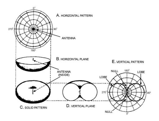
Figure 1-28.—Development of vertical and horizontal patterns.
