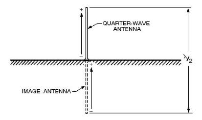
Figure 1-31.—Grounded quarter-wave antenna image.
