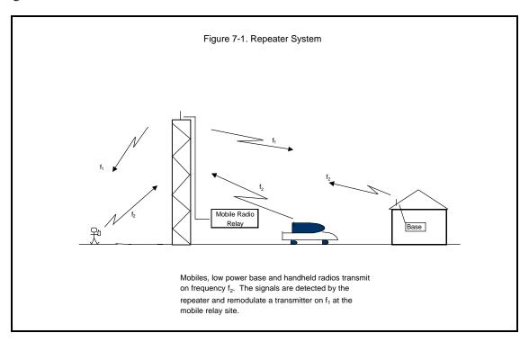
Twice the bandwidth of a simplex system is now required, further aggravating the spectrum efficiency problem. Voice FM simplex and repeater radio systems suffer from other disadvantages too. For example, when a base or repeater station is placed on a high point, it can cover distances of 60 miles or more in radius and thus, although not usually needed by the licensee, negates the option of relicensing the frequency to another user up to 120 miles from the licensee.
