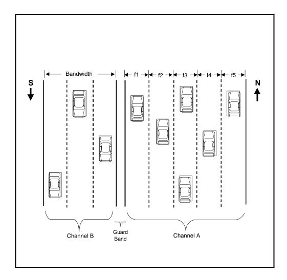
In a similar way, a second channel could be compared to the other side of the highway where all of the lanes travel in a different direction (southbound). A concrete barrier or median strip exists to separate the northbound lanes from the southbound lanes. A similar non-overlap space exists between channels and is called the *guard band*.
