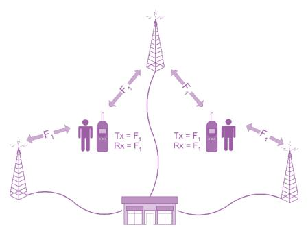
Figure 16-6: Simulcast Simplex Radio Example
