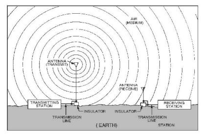
Figure 1-2.—Simple radio communication system.
