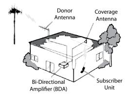
Figure 16-8:Bi-Directional Amplifier Example Source: PSWN. November 2002
