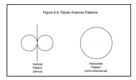
If the antenna is vertical to the earth's surface, its electric field will be vertical, and the antenna is said to have vertical *polarization*. If the antenna is horizontal and the electric field is parallel to the earth's surface, the polarization is horizontal. Almost all mobile operations use vertical polarization.
