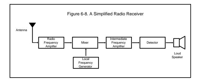
Radio systems are generally designed for AM or FM. Voice transmission is produced using a microphone at the input of the transmitter and a loud speaker at the output of the receiver. The signals are usually analog, or continuous, signals.
