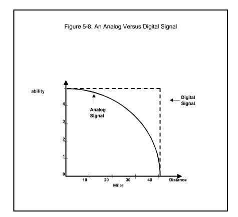
A comparison of the transmission differences between analog and digital signals is shown in figure 5-8.
