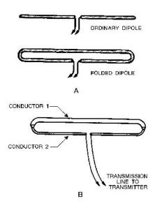
Figure 1-33.—Folded-dipole antennas.
