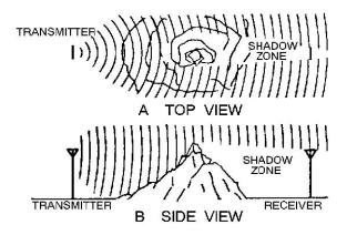
Figure 1-7.—Diffraction around an object.
