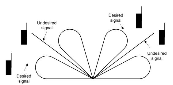
Figure 6-13. Pattern of Smart Antenna Adaptive Array
