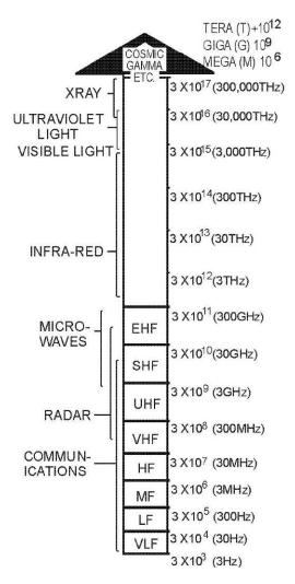
Figure 1-1.—Electromagnetic spectrum.
