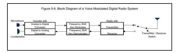
A digital radio system transmits data directly, by digitally modulating a carrier. One simple method of modulation is to change the carrier frequency by shifting it different amounts for each type of bit. (This is called *frequency shift keying*, or FSK.) The receiver then receives the signal as a zero or as a one and recreates the original signal.
