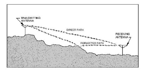
Figure 1-11.—Space wave propagation.
