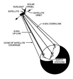
Figure 1-24.—Satellite/earth station communications system.
