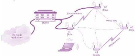
Figure 17-2: Mesh Networking of WLAN Access Points
