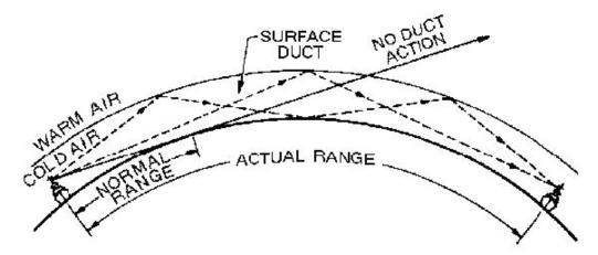
Figure 1-16.—Duct effect caused by temperature inversion.
