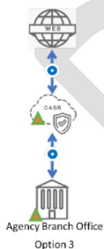
Through CASB or other SecAAS Bulk GRE/TLS, Client agent, proxy, etc.
