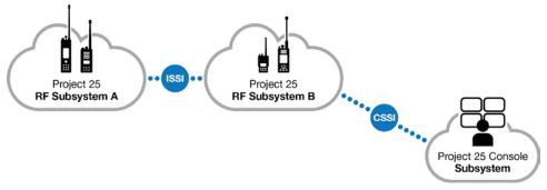
Figure 1 Connecting RF Subsystems Using ISSI and CSSI
