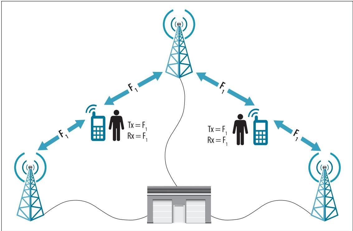
It's possible with conventional systems to simultaneously transmit the same signal from multiple locations. This is referred to as *simulcasting*. It requires careful synchronization of the individual transmitters and a healthy backbone of microwave or some other form of dedicated telecommunications circuit to deliver the outbound signal to all sites simultaneously.
