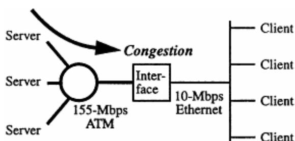
Congestion can also occur in a network node, such as a router or switch, from traffic aggregation in which traffic from multiple input ports is destined for a single output port. Traffic exceeding
