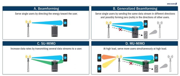
Figure 2. Advanced Antenna Systems - Beamforming and MIMO Examples<sup>16</sup>
