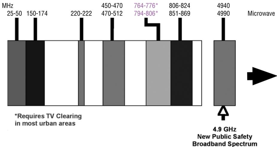
Figure 2-1: Radio Spectrum
