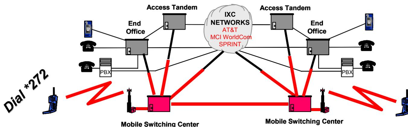
The diagram above is a representation of how the planned Wireless Priority Service (WPS) full operating capability (FOC) will work. The following is a brief description of how a WPS call will be processed.
