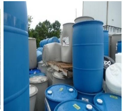
Chemical drums improperly stacked and some drums under duress.
