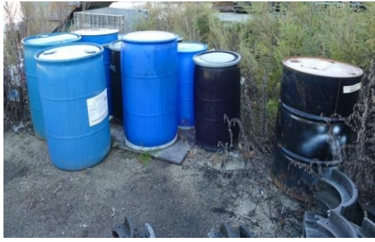
Chemical drums not properly labeled and no secondary containment.
