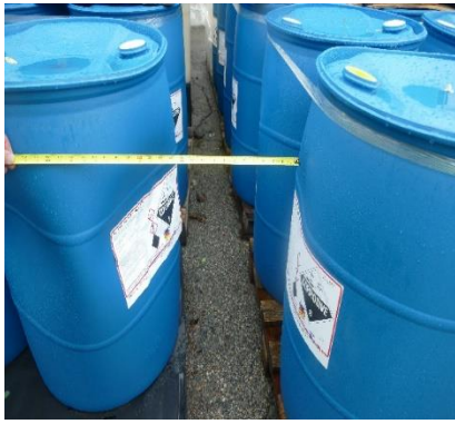
Insufficient aisle space between chemical drums.
